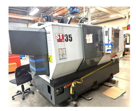
Haas CNC Control, 15" 3-Jaw Chuck, 12 Position Turret, Rigid Tapping Programmable Tailstock, tool setter, HIgh Intensity lighting High pressure coolant 300psi, chip conveyor, remote jog handle
