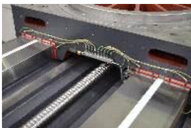
Specific Box Ways – X Axis (on the Left), Z Axis (in the Middle), Y Axis (on the Right) with Way Lubrication
