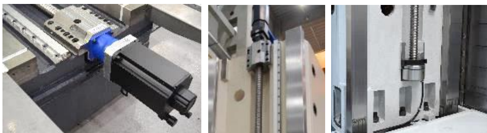
An Example of Placing of the Ball Screw on the X and Y Axes
