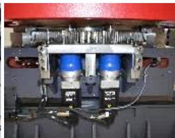
Rotary Table – B Axis Drive, Two Servomotors in the Master-Slave Function (in the Middle) and a Cross Bearing Installation (on the Right)
