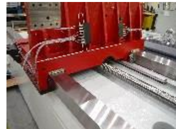
Specific Box Ways – X Axis (on the Left), Z Axis (in the Middle), Y Axis (on the Right) with Way Lubrication
