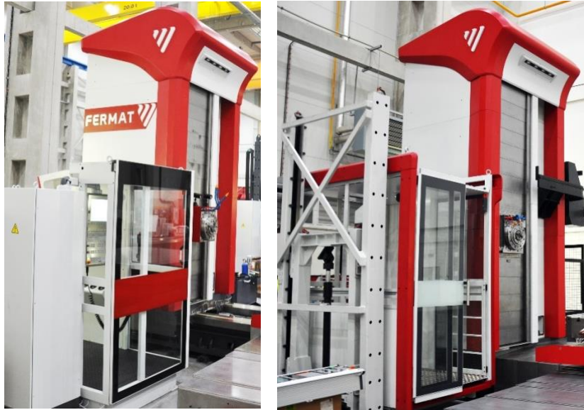
illustrative pictures: fixed shield opened from the back, no travel (left), movable cabin (right)
